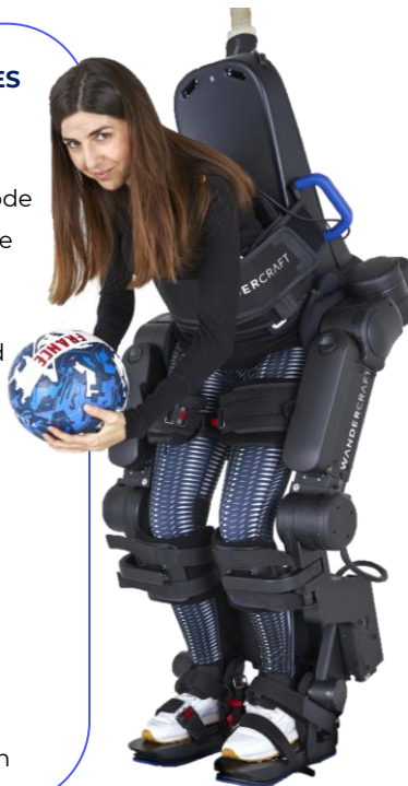
Figure 1. Tetraplegic patient during training with the Atalante exoskeleton (Wandercraft, France)
