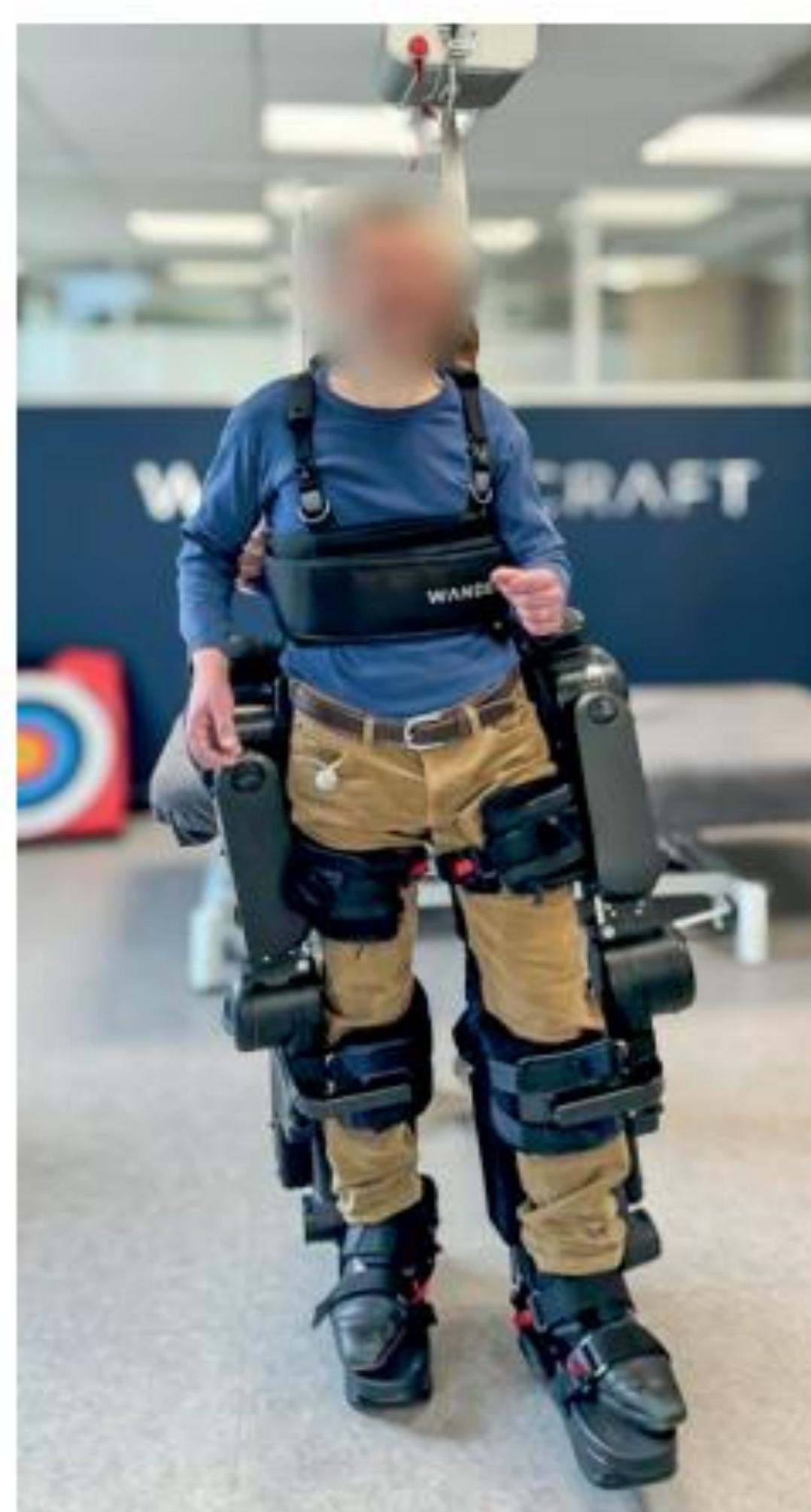
Figure 2. Illustration of the hands-free Atalante X exoskeleton in use
